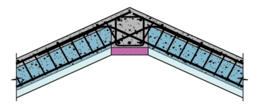
Section Through An ICF Roof Deck Showing Tee-beams
