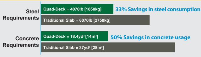
By reducing your Steel & Concrete Requirements with Quad-Deck, you also reduce your Mass by over 50% and use 50% less Shoring.
